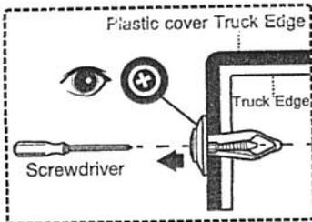
Remove 6 plastic pooks follow diagram using screw driver.
