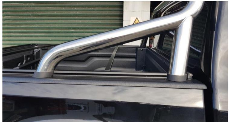
7. With 2 people hold firmly on each side rail so the cross-bar is not loose. Make sure both side rails have the same gap from the edge of the inner bed liner to the side rail) and with the 3mm drill bit mark the Bed liner through the pre-drilled holes in the side rails. Remove the rails and drill the holes through bed liner and wellside.
