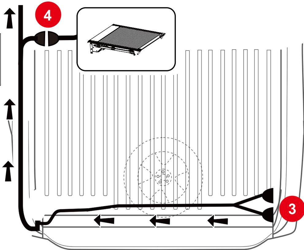
CONNECTION OF Y-SOCKETSIGNAL WIRING FORM CENTRAL LOCK (POINT 3) TO E-ROLLER LID UNIT (POINT 4)
