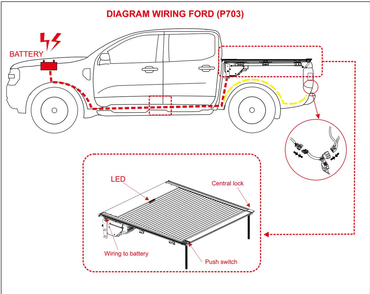
E-roller lid to follow to the main chassis wiring harness
