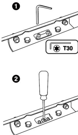
1. Remove the 2 pcs screws and fixing plate in following picture with T30
