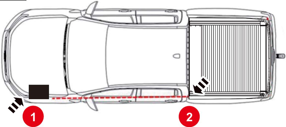
WIRING BATTERY (POINT 1) TO E-ROLLER LID (POINT 2) BY WIRE HARNESS BATTERY RKE
