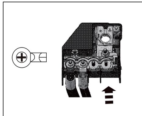
Apply nut to lock ring connector and battery electrode with Torque 10Nm+/- 1.5Nm
